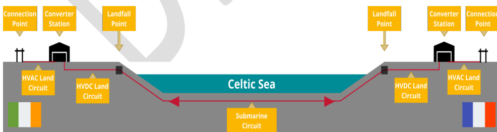
Figure 2.1: Celtic Interconnector Overview of Project Elements (Source: EirGrid)
